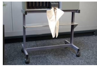
Option: The trolley is a simple solution to place the PRC 410 in an ergonomically suitable height and allows easy movement of the machine.
