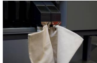
Coin bagging attachments can be easily interchanged with the coin drawers – up to 8 at 1 time
